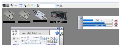
After add and finishing setting up step,press ico (save as) jumps out of the following window fill in the document needing to preserve, at the same time choose jadd to cue; frame ,press the button of jsave to preserve it ,and then exit.
