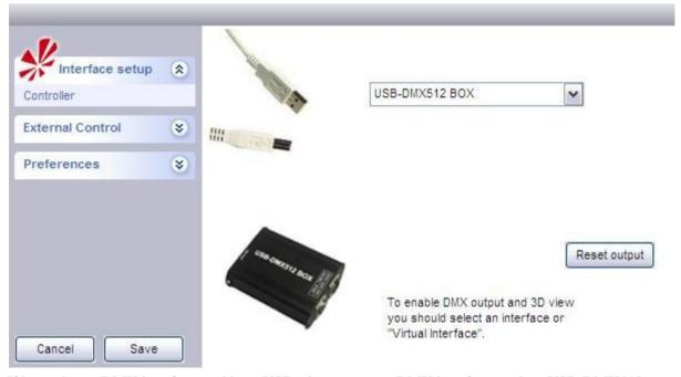
If have chosen DMX interface, and have USB wire to connect DMX interface, such as USB-DMX512 BOX interface, reset FreeStyler software, when schedule bar process to 80%, if the green LED light of interface bright, means the software recognize the interface, DMX signal could output at this moment.
